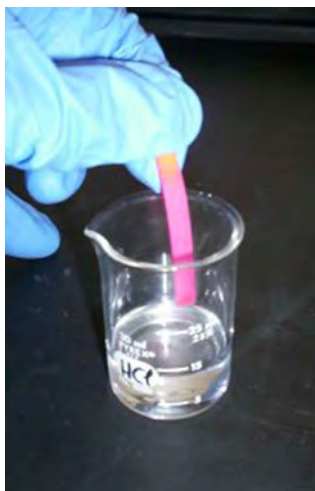
Figure 6.42 The pH of hydrochloric acid is tested with litmus paper. (credit: David Berardan)
