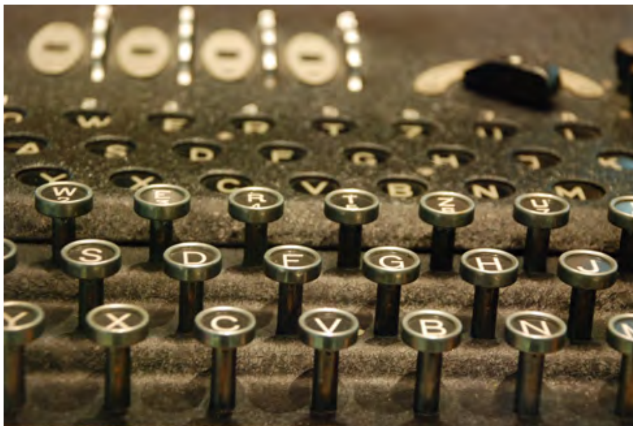
Figure 11.1 Enigma machines like this one, once owned by Italian dictator Benito Mussolini, were used by government and military officials for enciphering and deciphering top-secret communications during World War II. (credit: Dave Addey, Flickr)
